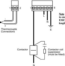
Note to ensure compliance with the EMC & LVD Directives lead lengths should not exceed 3m.
