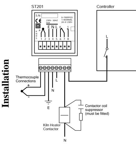
A basic wiring scheme is shown above. A better scheme is to use the ST201 to control a secondary contactor. The power contacts for the two contactors are wired in series. This scheme guards against the possibility of the kiln heater contactor failing closed. Some controllers have a secondary output which is deenergised if the controller detects an over-temperature condition. Wire this output to a secondary contactor via the ST201 contacts. Note that the ST201 contacts are volt-free.
